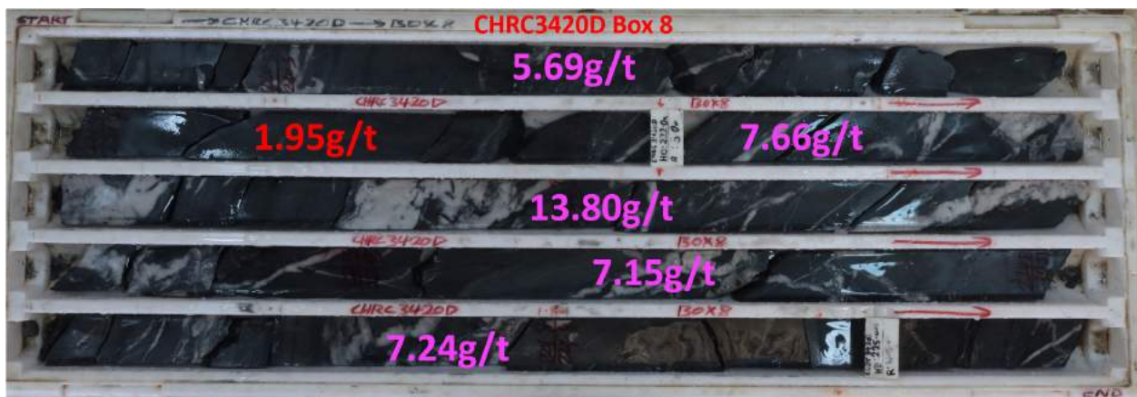
Figure 4: Drill Core photo of high-grade gold in vein hosted metasedimentary unit.
