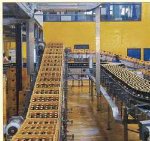
The world class packaging line, to be commissioned in November 2003, increasing capacity to 40,000 bottles per hour
