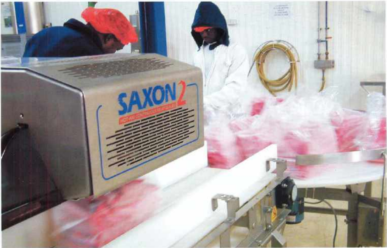
Sealing of Fanyogo product bags with a Saxon 2 Heat Sealer.
